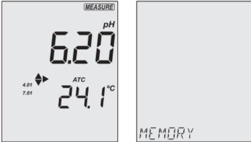
2. Press MR to recall the last recorded pH, ORP, temperature and calibration values.
