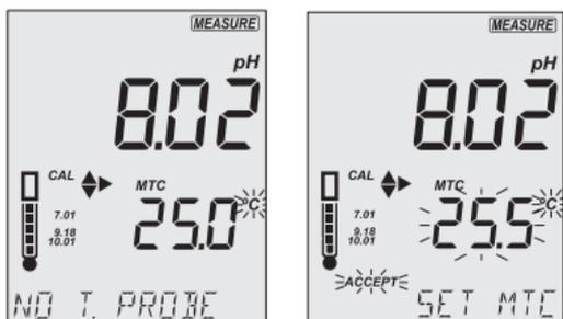
**Note:** The temperature value used for MTC can be set only when "NO T. PROBE" message is displayed.
