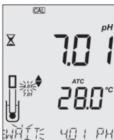
For one-point calibration, press CAL/EDIT to exit calibration. The meter stores the calibration and returns to Measurement mode.
