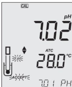
2. When the reading is stable and close to the selected buffer, the ACCEPT tag is displayed blinking. Press GLP/ACCEPT to confirm calibration.
