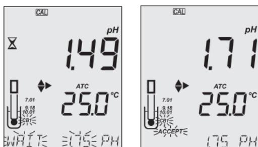
**Note:** When using custom buffers, CB1 and CB2 tags are displayed. If only one custom buffer is used, CB1 is displayed together with its value.
