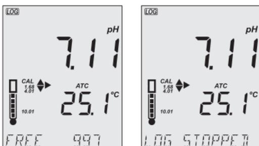
4. Press LOG/CLEAR again (or ESC) to end current interval logging session. LCD displays "LOG STOPPED". Meter returns to measurement screen.
