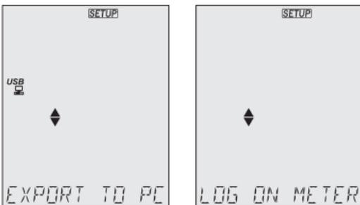
**Note:** This option is only available while connected to a PC. The USB/PC icon is not displayed if LOG ON METER option was previously set.
