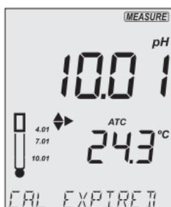
If the instrument is not calibrated or calibration has been deleted, the “NO CAL” message is displayed.
