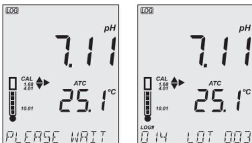
3. Press RANGE/▶ during logging to display the number of available records ("FREE" ###). Press RANGE/▶ again to return to return to active logging screen.
