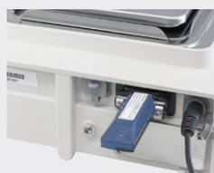
*AD-8529PC-W interface to PC with USB port up to 10m distance*
